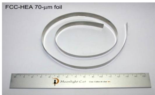
Fig. 1. A roll foil 70 \mu\text{m} thick from the \text{Al}_5\text{Cr}_{12}\text{Fe}_{35}\text{Mn}_{28}\text{Ni}_{20} alloy obtained by arc melting and cold rolling (the elongation in rolling is 4.257 % depending on a blank with the initial thickness of \sim 3 mm and hardness of 147 HV [13; 23])
